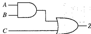
(b) Logic circuit based on Karnaugh map
